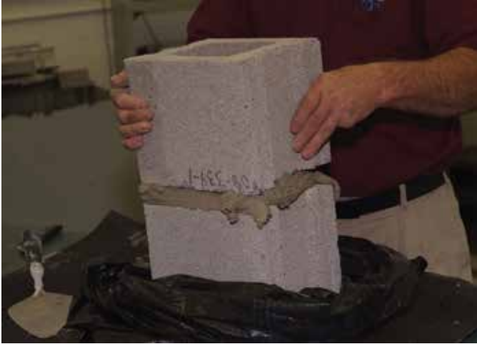
Fabrication of an 8 x 8 in. (200 mm) block prism per ASTM C1314, Standard Test Method for Compressive Strength of Masonry Prisms
