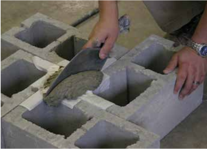
Proper use of CMUs to fabricate a compressive strength test specimen, per ASTM C1019, Standard Test Method for Sampling and Testing Grout
