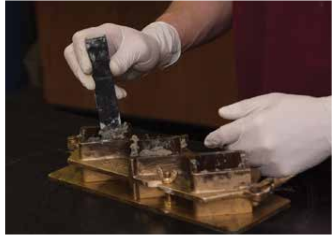
Casting of mortar cubes per ASTM C109, Standard Test Method for Compressive Strength of Hydraulic Cement Mortars (Using 2-in. or (50-mm) Cube Specimens)
