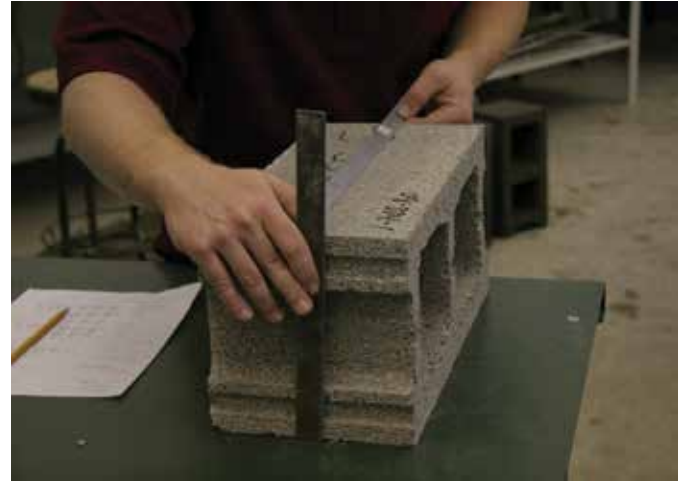
Checking dimensional requirements of a CMU per ASTM C140, Standard Test Methods for Sampling and Testing Concrete Masonry Units and Related Units
