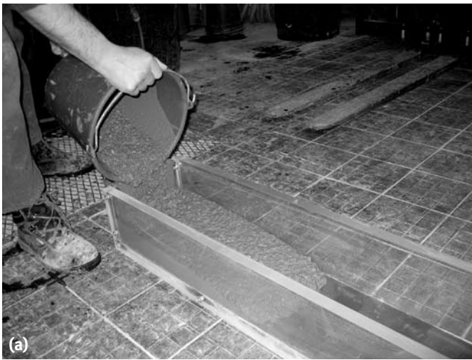
Fig. 2: The LCPC Box test for SCC: (a) the SCC is slowly poured into the box at one end; and (b) correlation between measured spread length and a yield stress of the tested material (1 in. = 25.4 mm, 1 psi = 6890 kPa)
