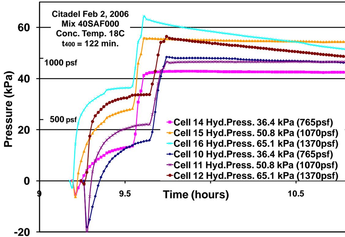
**Figure 3 – Typical replicate lateral pressure measurements.**
