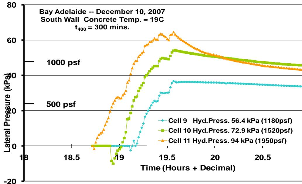
Figure 13 – Typical pressure results for South wall
