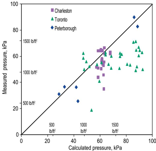
Fig. 9: Comparison of measured and predicted lateral pressures (1 kPa = 21 lb/ft<sup>2</sup>)
