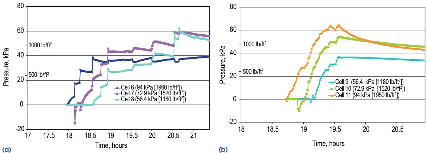
**Fig. 8: Lateral pressure versus time from start of data logger for Bay-Adelaide, Toronto, ON, with concrete temperature of 19°C (66°F): (a) North wall, and (b) South wall. Hypothetical hydrostatic pressures are provided in the legends**
