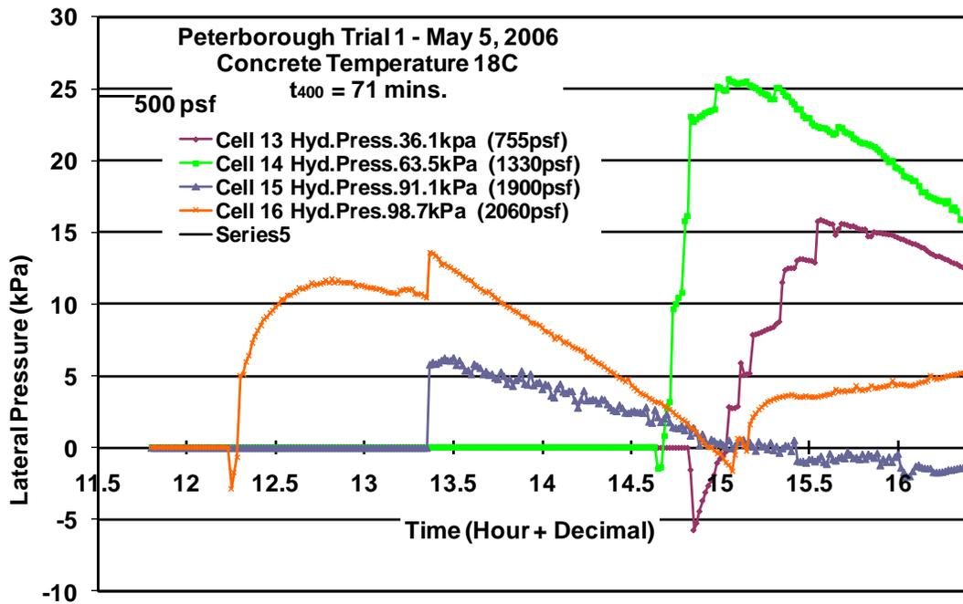
**Figure 7 – Lateral pressure measurement Peterborough Mixture 1**
