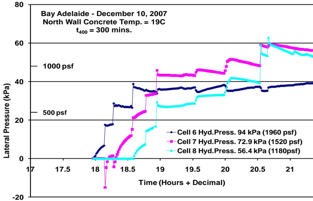
Figure 12 – Typical pressure results for North wall
