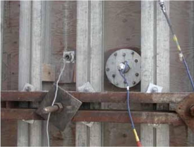
Fig. 1: Geokon 4820 earth pressure cell at Peterborough, ON, site
