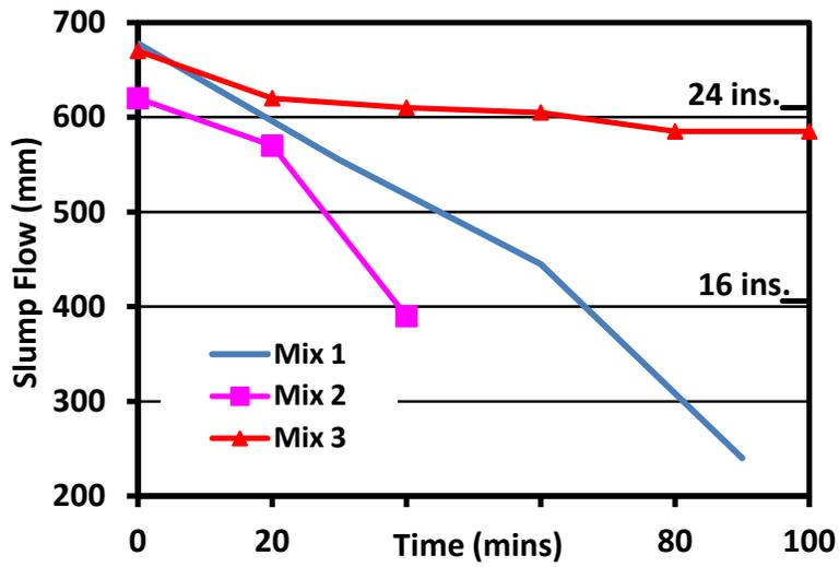
**Figure 6 - Slump flow loss (Peterborough mixes)**
