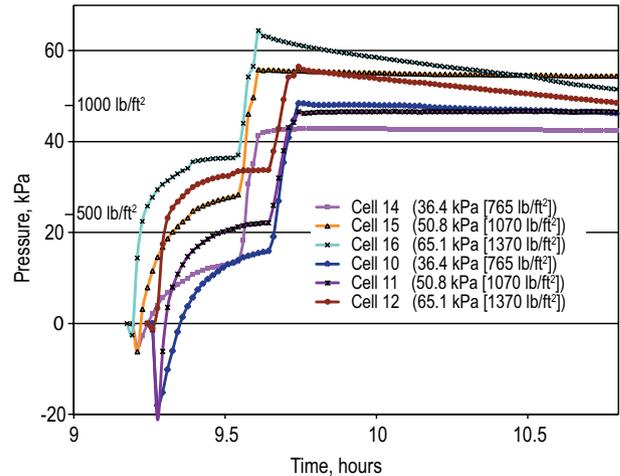
Fig. 3: Lateral pressure versus time from start of data logger for Citadel, Charleston, SC, with concrete temperature of 18°C (64°F) and mixture  $f_{400}$  of 122 minutes. Hypothetical hydrostatic pressures, based on fluid head above each cell, are provided in the legend
