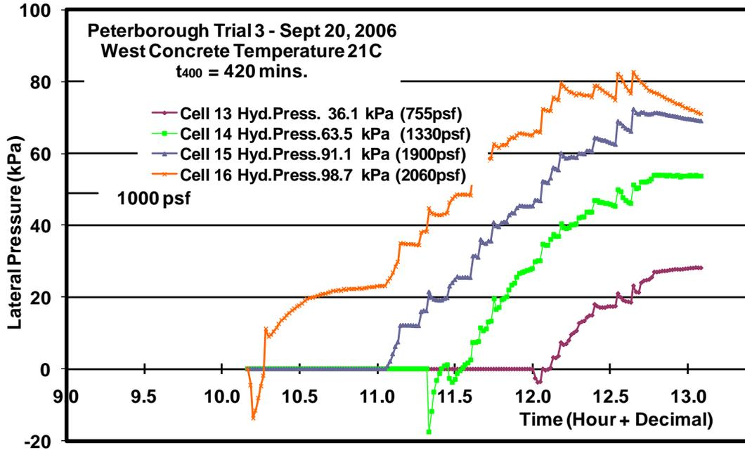
**Figure 9 – Lateral pressure measurement Peterborough Mixture 3**
