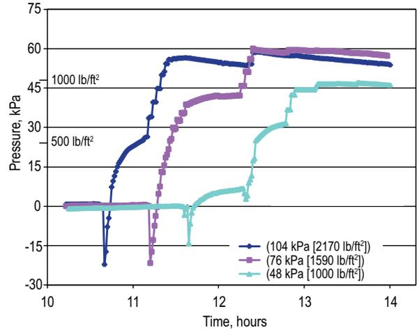
Fig. 5: Lateral pressure versus time from start of data logger for Labatt's Brewery, London, ON, with concrete temperature of 17°C (63°F). Hypothetical hydrostatic pressures are provided in the legend
