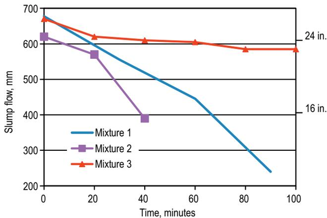
**Fig. 6: Slump flow loss for mixtures for Regional Hospital at Peterborough, ON, site (1 mm = 0.04 in.)**
