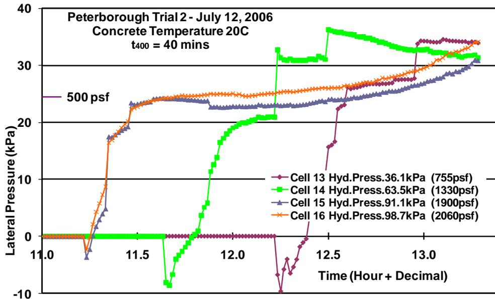
**Figure 8 – Lateral pressure measurement Peterborough Mixture 2**
