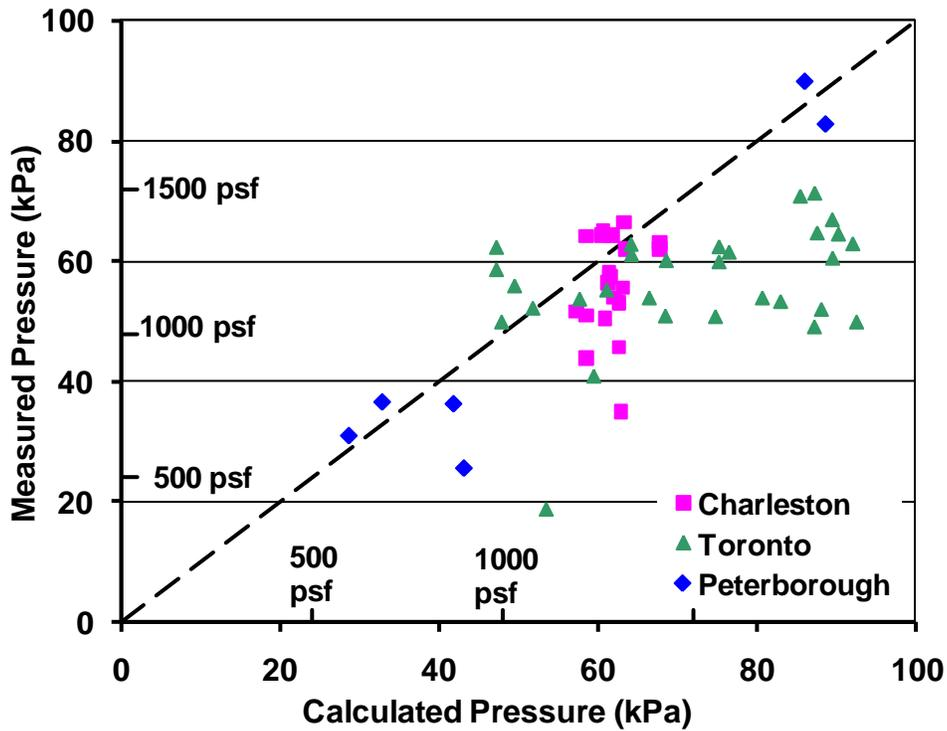
Fig 14 - Comparison of Measured and Predicted Lateral Pressures
