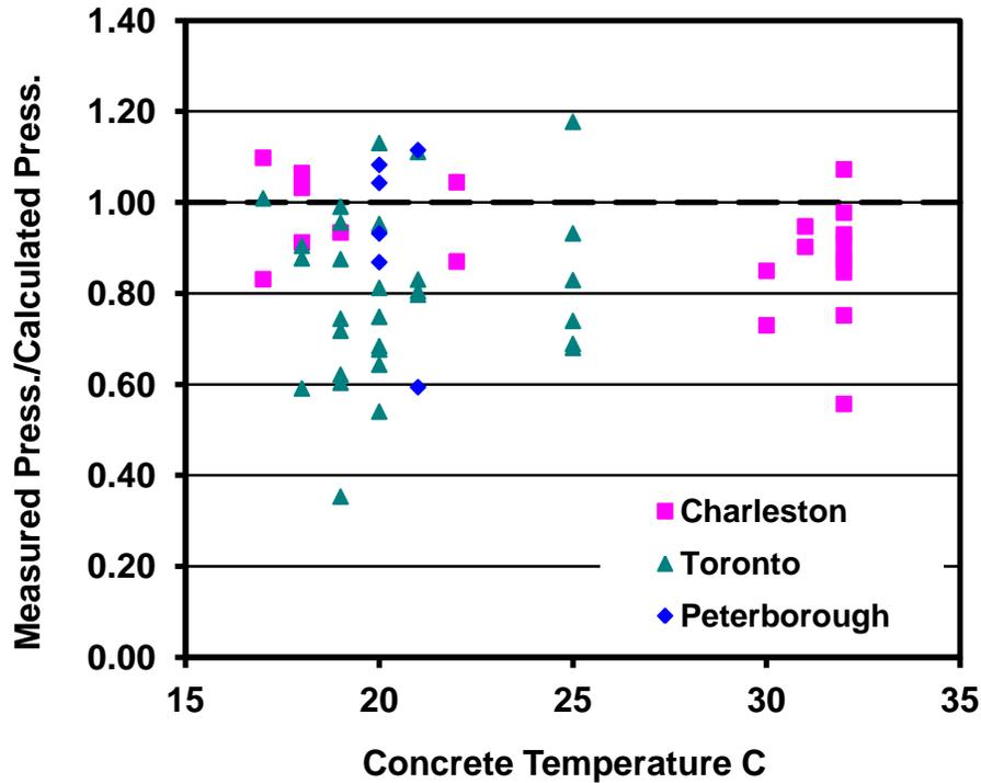
**Fig 15 – Sensitivity of Measured/Predicted Lateral Pressures with Concrete Temperature**
