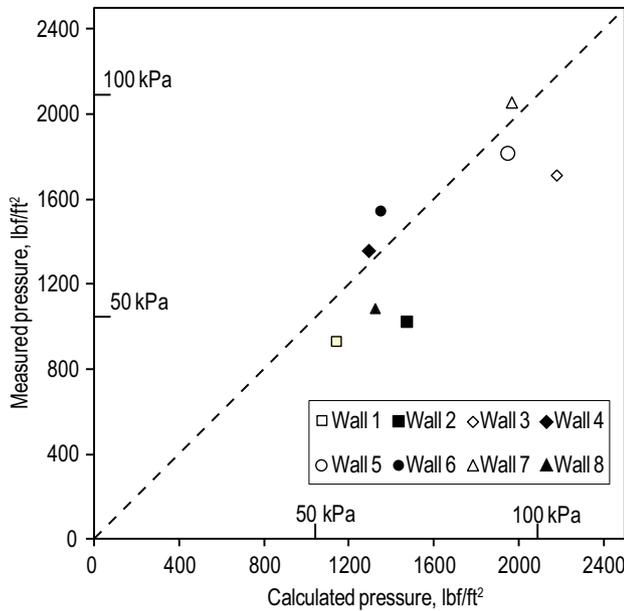
Fig. 4: Comparison of the maximum pressures measured in TC 233-FPC test program in Stockholm with maximum pressures predicted by Eq. (4)
