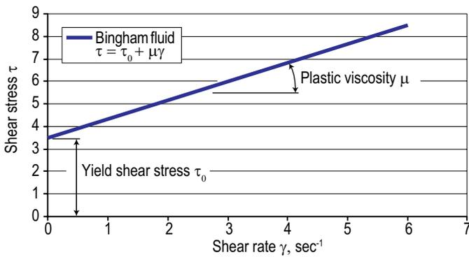
Fig. 1: A Bingham fluid is capable of resisting a statically applied shear strain up to a limiting (yield) stress. With increasing strain rate, the material’s resistance to shear stress increases in proportion to its plastic viscosity
