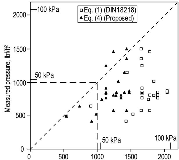
Fig. 5: Comparison of values calculated using Eq. (1) and Eq. (4) with pressures measured on tall forms
