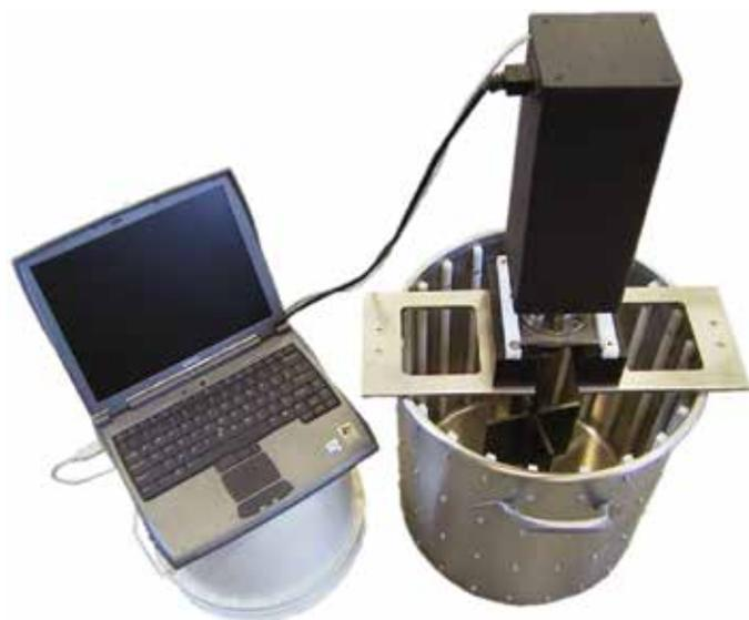
Fig. 2: Typical, commercially available portable rheometer
