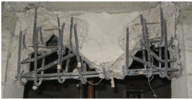
(a) Specimen CW-1: Typical beam damage (2 nd floor beam pictured)
