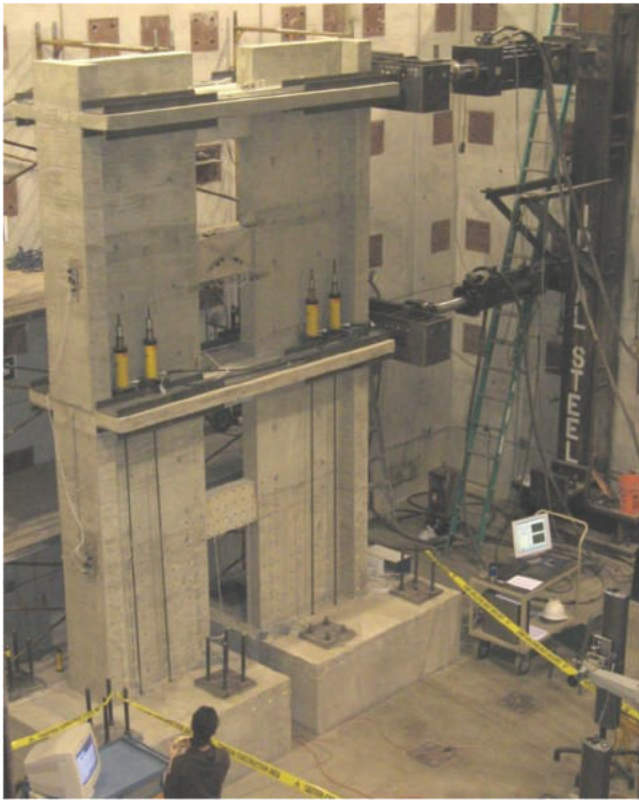
Fig. 1—Coupled wall specimen, before testing.
