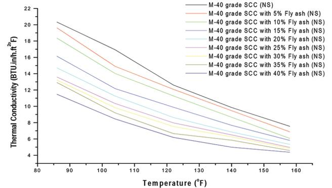
Variation of Thermal Conductivity (*k*) with Temperature for M-40 grade SCC (CS)
