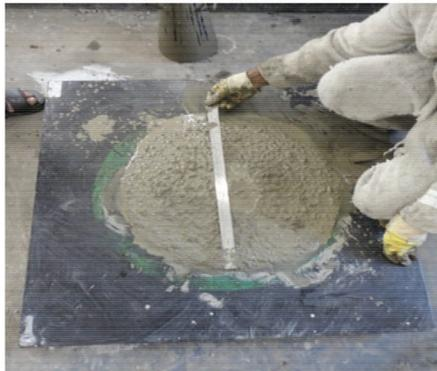
Slump Flow for M-40 grade SCC (CS)
