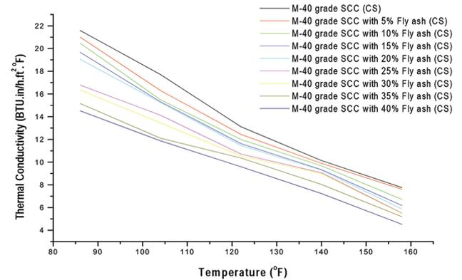
Fig. 8—Variation in *k* value with temperature for various concrete mixtures. (Note: 1 BTU.in./h.ft<sup>2</sup>.°F = 0.1442 W/m°C.)
