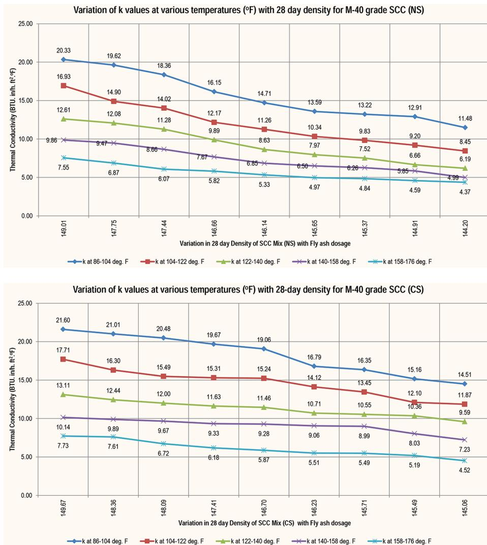
Fig. 7—Variation of  $k$  value with 28-day density of concrete mixture at various test temperatures. (Note:  $1 \text{ BTU.in./h.ft}^2.\text{°F} = 0.1442 \text{ W/m}^2\text{.°C}$ ;  $\text{°F} = (\text{°C} \times 9/5) + 32$ .)
