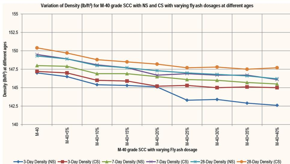
Fig. 4—Variation in density of M-40 grade SCC with NS and CS with varying fly ash dosages at different ages. (Note: 1 lb/ft<sup>3</sup> = 16.02 kg/m<sup>3</sup>.)
