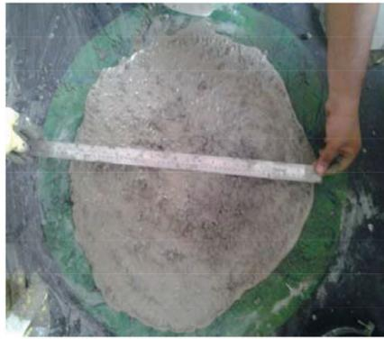
Slump Flow for M-40 grade SCC (NS)
