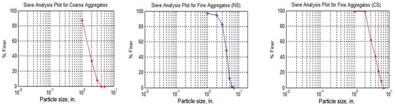
Fig. 3—Sieve analysis plots for coarse and fine aggregates. (Note: 1 in. = 25.4 mm.)
