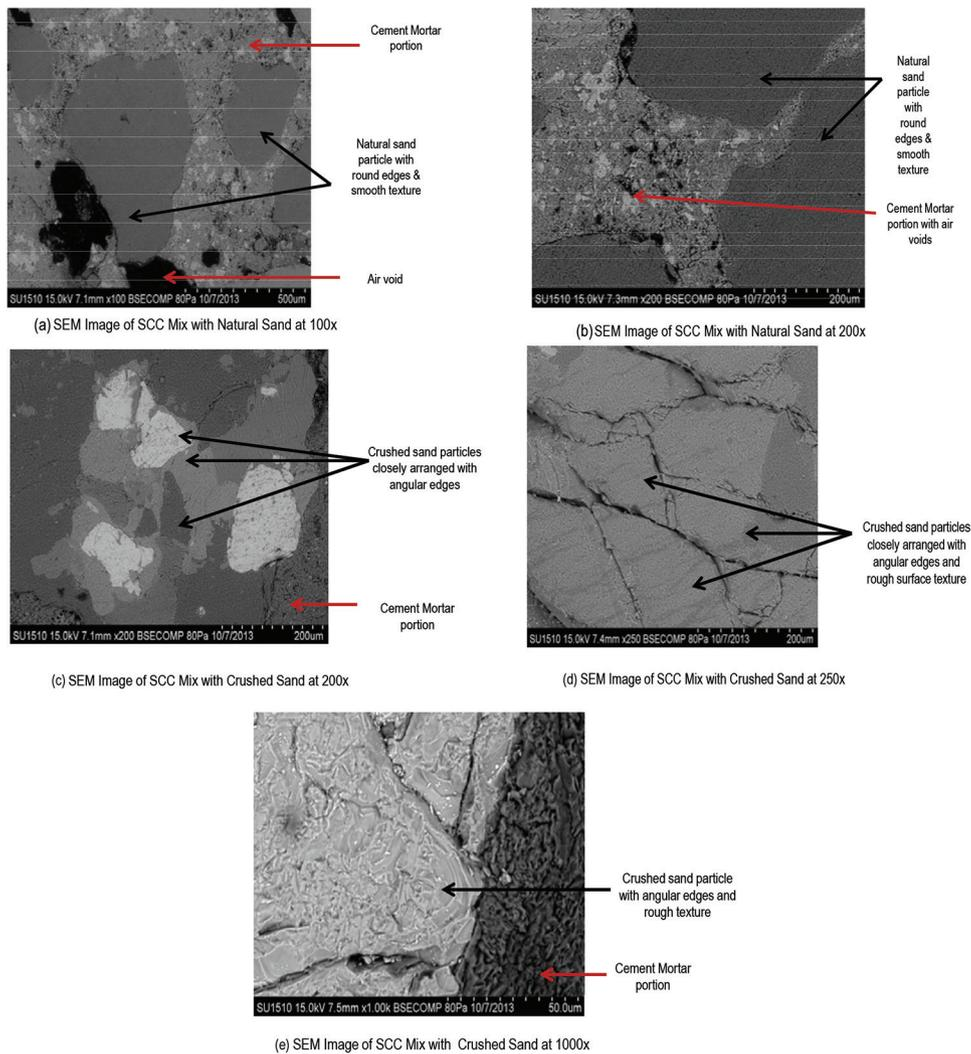
Fig. 1—SEM images of M-40 grade SCC with NS and CS at various magnification levels.
