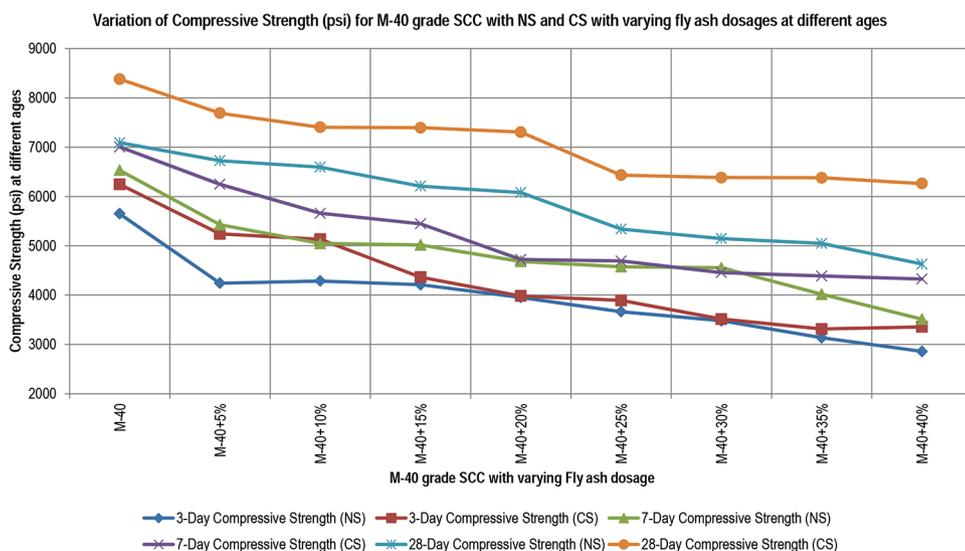
Fig. 5—Variation in compressive strength of M-40 grade SCC with NS and CS with varying fly ash dosages at different ages. (Note: 1 psi = 6.895 × 10<sup>-3</sup> MPa.)
