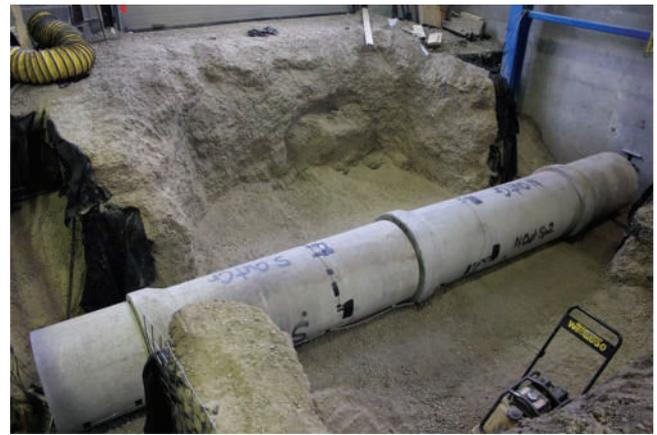
Fig. 4—0.6 m (24 in.) diameter pipes before burial with Class IV pipe on the right and Class V pipe on the left.
