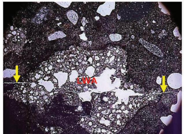
4b. Plane-polarized light photomicrograph showing microcrack that cut through LWA. Length of field of view from left to right is 2 mm.
