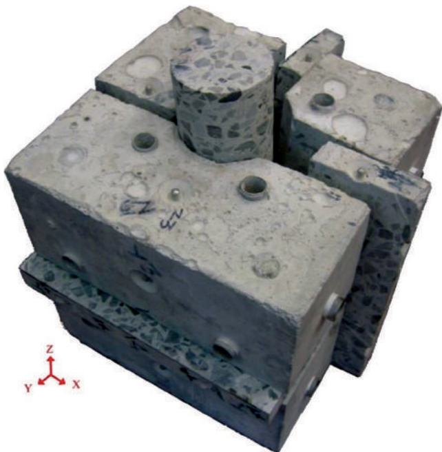
Fig. 2—Dissection of no-stress cube specimen (254 mm [10 in.] size) along three mutually perpendicular planes (YZ, ZX, and XY) for DRI analysis and core-drilled along Z-axis.
