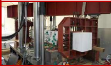
Beam Torsion Test
