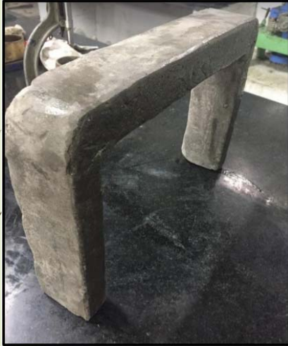
Fig 2 Finished arch after curing
