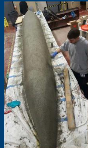
Touched up the end caps with concrete mix then proceeded to smooth out the concrete
