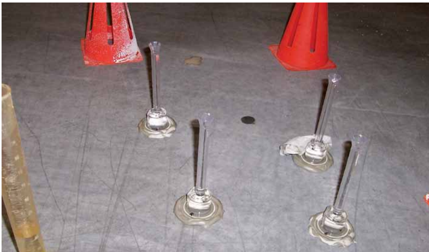
Fig. 2: Testing for relative absorption using Rilem tubes. In this case, four tubes were used at each test site/cycle
