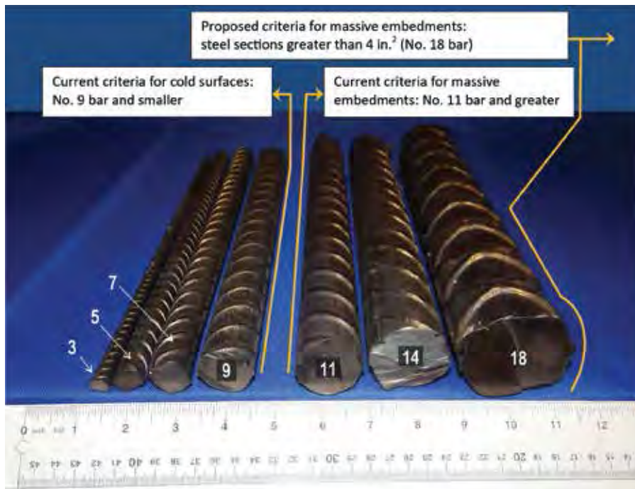
Fig. 4: Massive embeddings are currently classified as steel sections larger than a No. 9 bar. Based on recent findings, 6 it is recommended that the massive embedding classification be increased to steel sections larger than a No. 18 bar (4 in. 2 (2500 mm 2 ) cross-sectional area)
