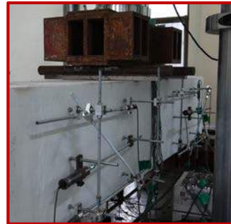
Beam Shear Test
